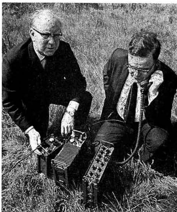
The Redifon GA480 linear amplifier and GR345 s.s.b. manpack undergoing a "field" demonstration in the hands of R. Vaughan, G3FRV (right) of the development team and K. E. Harris, Executive Director of Redifon Ltd.
